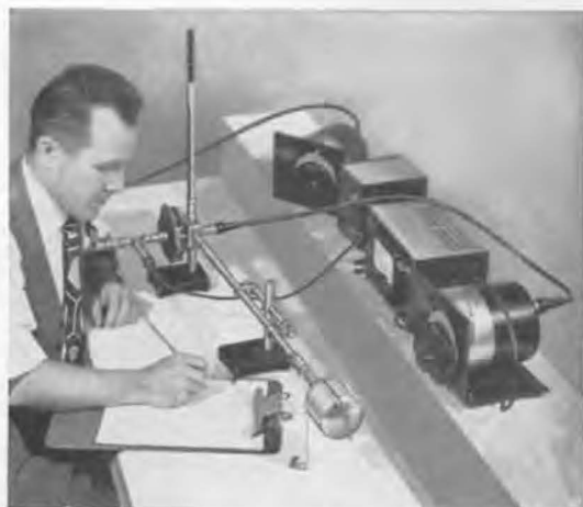
Type DNT Detector is recommended for use with the Type 1602-B UHF Admittance Meter and is shown here with the Admittance Meter in the measurement of resistors at 800 Mc.
