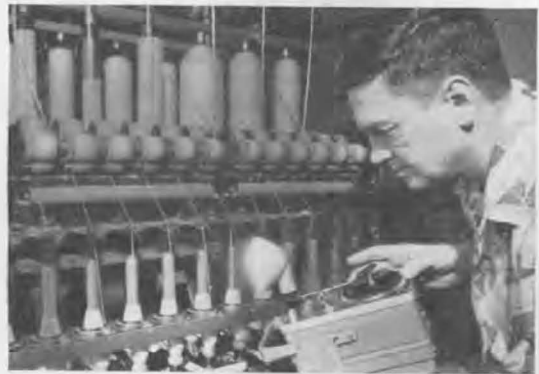
Under a stroboscope's light, the fast action of textile machinery is frozen for inspection or for speed measurements.
