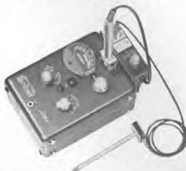
The vibration pickup and control box plug into the Sound-Level Meter in place of the microphone. The control box fastens to one end of the Sound-Level Meter, as shown above.
