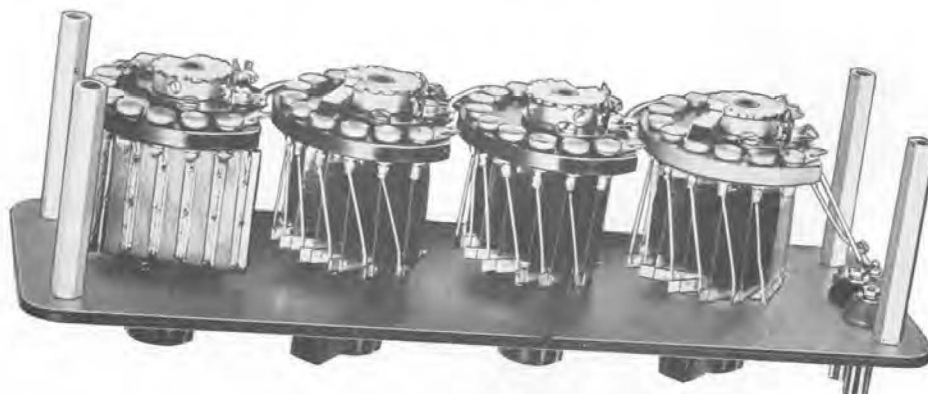
Interior view of Type 1432-Q Decade Resistor
