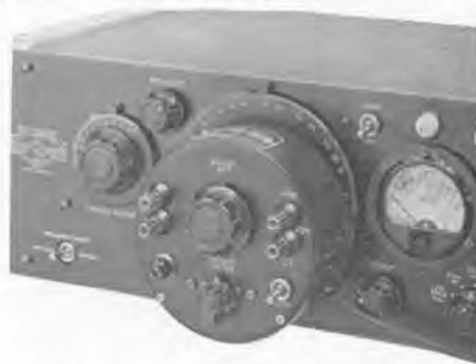
Type 1304-B Generator driven by a Type 908-R Dial Drive, for use with an X-Y plotter.
