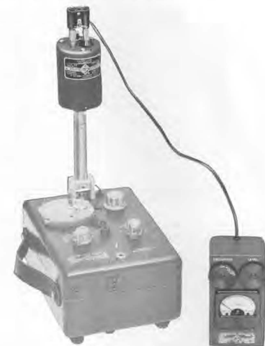
Calibrator fits over Microphone of Type 1551-C Sound-Level Meter. At right is Type 1307-A Transistor Oscillator.
