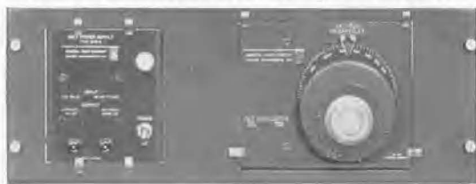
Unit Oscillator with Unit Power Supply in Relay-Rack Adaptor Panel.
