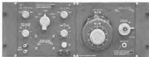
Oscillator with Modulating Power Supply and Panel Extensions for relay-rack mounting.
