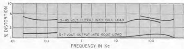
Typical output and harmonic distortion characteristics of the Type 1210-C Unit RC Oscillator as functions of frequency and load.
