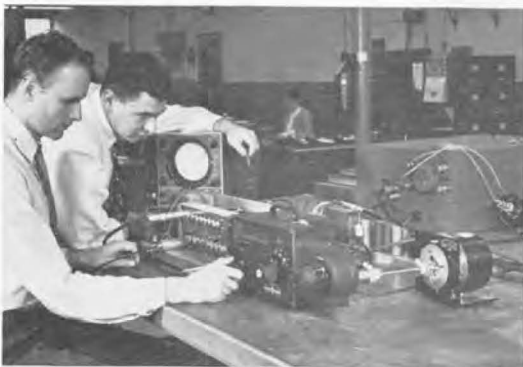
General Radio Sweep Drive and Unit Oscillator used in the test of wide-band amplifiers.
