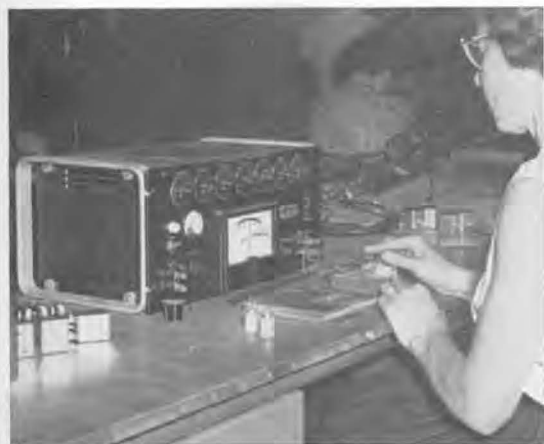
Resistance Limit Bridge used to test relay coils for precision relays and switches.
