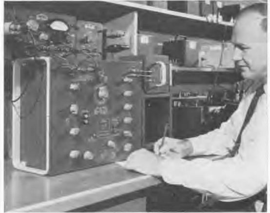
The Type 1632-A Inductance Bridge is shown in a laboratory set-up for the measurement of standard inductors.
