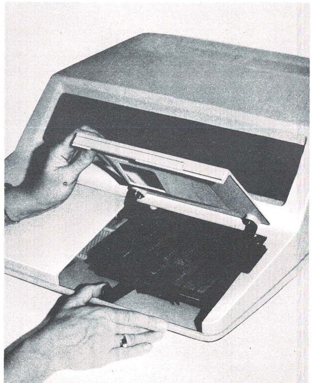
Installing a program board.
