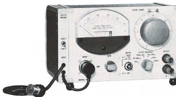
1232-P2 Preamplifier installed.
