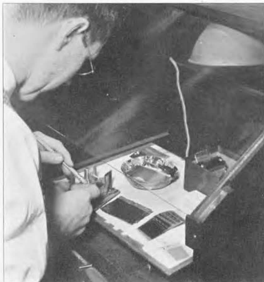
(Left) Assembling sheets of mica and foil into TYPE 505 Condensers. The assembly operation is carried out under a glass cover to protect the condensers from dust, and the foil and mica are kept on an electrically heated plate to prevent moisture from condensing on their surfaces.
