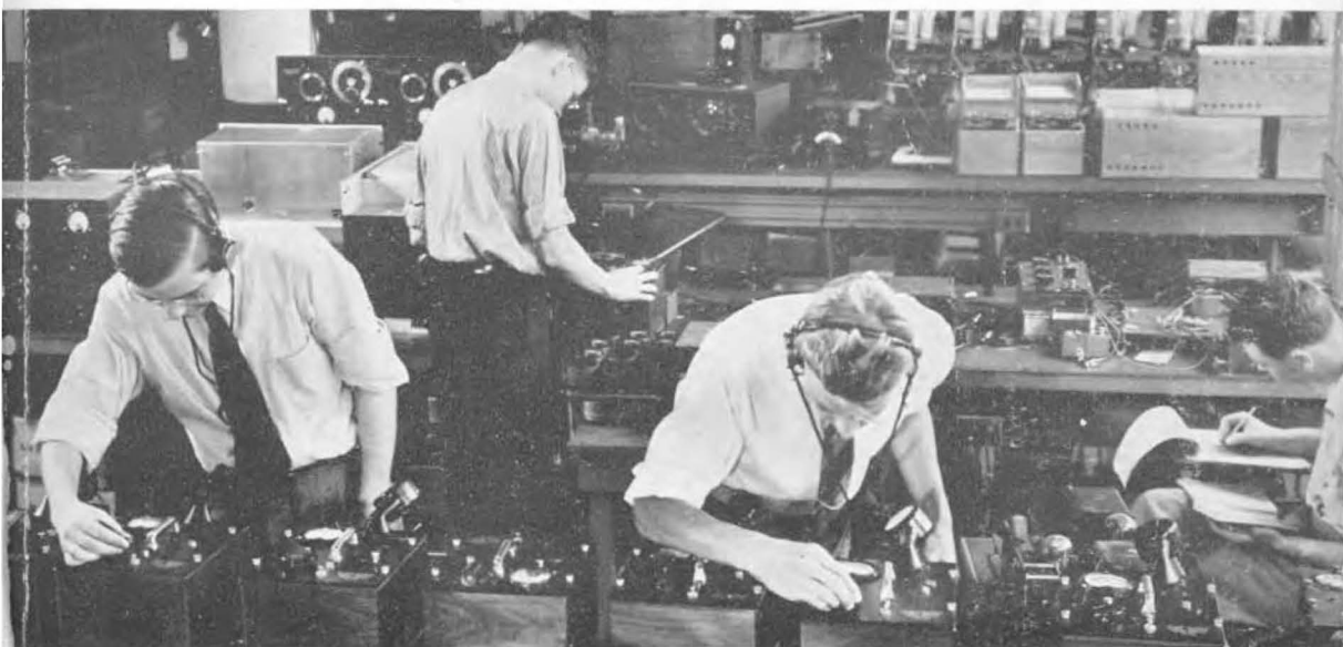
Above—Calibrating Type 724-A Precision Wavemeters in the standardization laboratory. Below—Analyzing fan noise with the Type 760-A Sound Analyzer.
