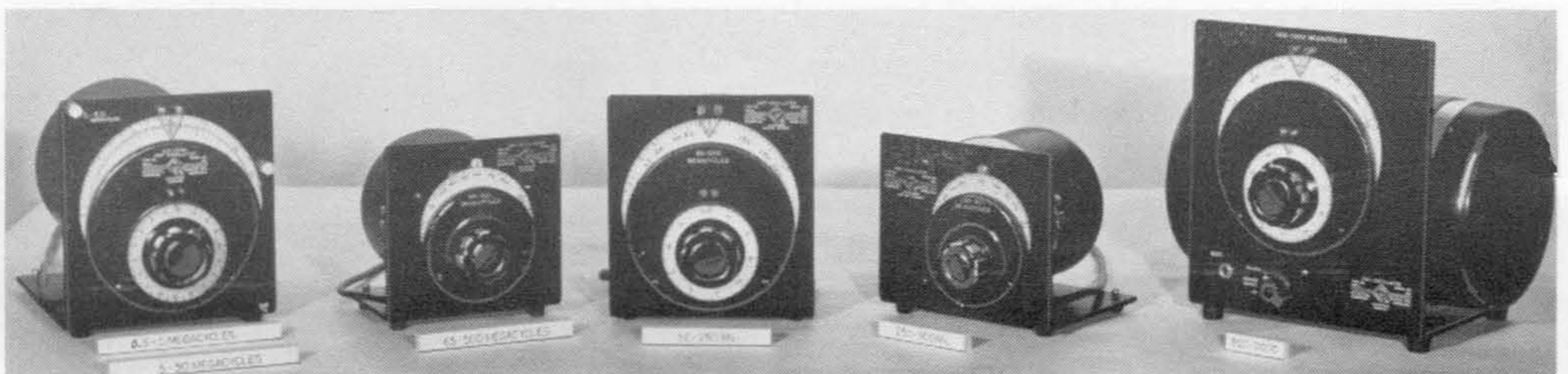
Figure 2. Group of Unit Oscillators covering a frequency range of 0.5 to 2000 megacycles. The lengths of the bars in front of the units indicate their frequency coverage on a logarithmic scale.
