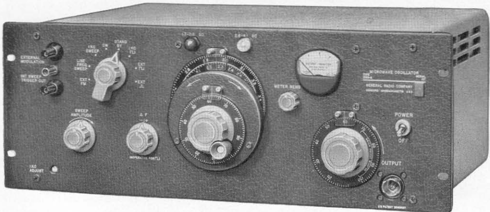
Figure 1. Panel view of the Microwave Oscillator.
