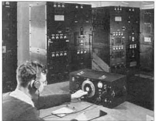
This view shows the TYPE 620-A Heterodyne Frequency Meter and Calibrator in use in a radio-telegraph station. The cabinet model shown is particularly useful for marine work since it can be used both in shore stations and on shipboard and with either a-c supply or batteries.
