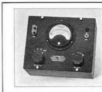
TYPE 487-A Megohmmeter, a direct-reading instrument operating on the ohmmeter principle, is described on page 123.
