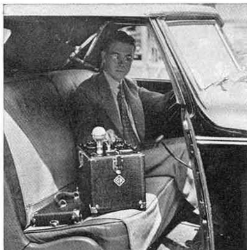
This photograph shows the TYPE 759-A Sound-Level Meter used to measure automobile noise.
