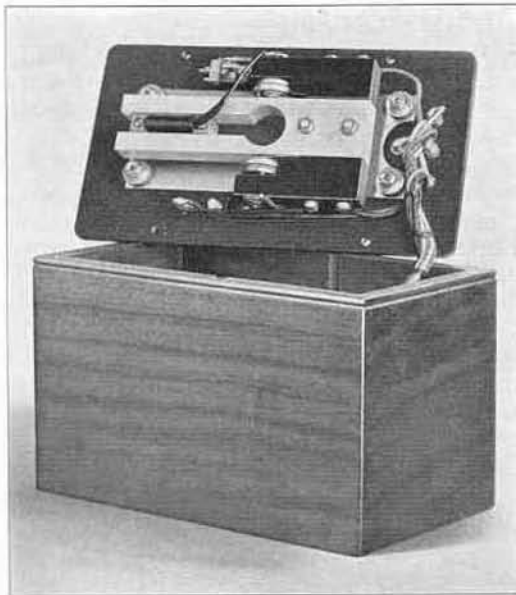
View of the interior of TYPE 813-A Audio Oscillator showing the tuning fork and its mounting. Inside the cabinet are a filter and an output transformer.
