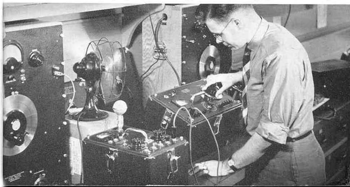
Above—Calibrating Type 724-A Precision Wavemeters in the standardization laboratory. Below—Analyzing fan noise with the Type 760-A Sound Analyzer.
