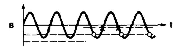
Figure 2-7b. Too large a negative offset of the TRIGGER LEVEL control. Corrected by reducing offset.
