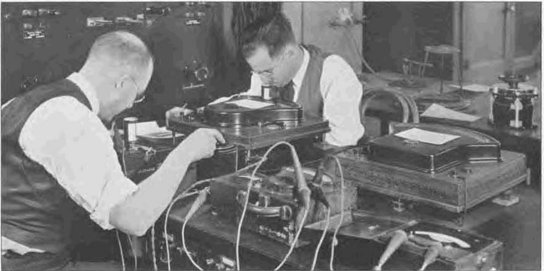
Standardizing meters with the aid of VARIACS in the laboratory of a public utility company.
