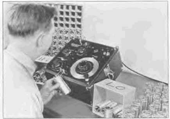
Production testing of electrolytic condensers with the capacitance test bridge.
