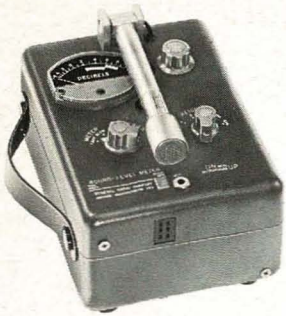
(Left) Microphone in the storage position (batteries automatically disconnected). (Center) The sound-level meter operated in its leather carrying case, microphone in the horizontal operating position. (Right) The sound-level meter ac-operated with the Type 1262-B Power Supply, which plugs directly into the base of the sound-level meter.
