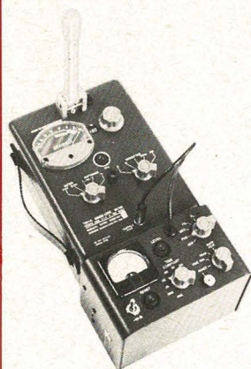
The 1556-B Impact-Noise Analyzer attaches to the 1551-C Sound-Level Meter as shown here.
