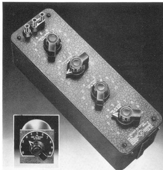
Figure 1. View of a Type 1432-A Decade Resistor. Inset at lower left shows Type 510-D Decade-Resistance Unit.
