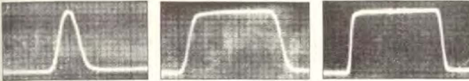
Output pulse waveforms 20-cps to 3-Mc range; input-pulse rise time, 0.03 \mu sec; three pulse lengths shown.
