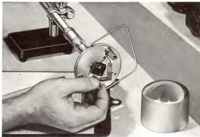
The Type 874-ML Component Mount is shown here attached to the Type 874-LK20L Constant-Impedance Adjustable Line. These useful accessories plug easily into the Admittance Meter. Also shown is the Type 874-Z Stand, which provides support.
