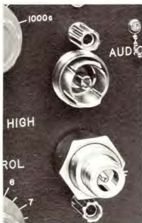
locking Type 874 panel connector adapted to type N with Type 874-QNJL
