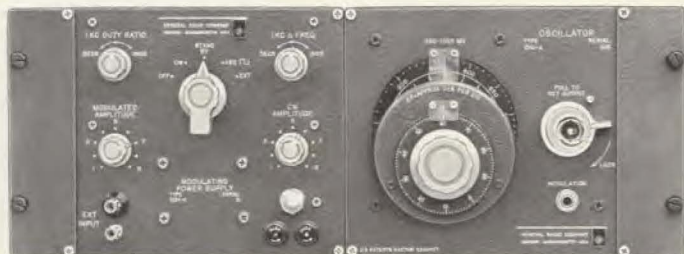
The Type 1361-A UHF Oscillator and Type 1264-A Modulating Power Supply assembled with Type 480-P416 Adaptor Plate Set for rack mounting.
