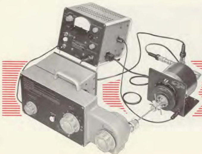
A constant-amplitude sweeping system, consisting of a Unit Oscillator, sweep drive (page 127), amplitude-regulating power supply, voltmeter rectifier (page 67), patch cord (Type 874-R22A, page 71), and tee (page 72). When a 50-ohm system is being measured, use Type 874-VQ Voltmeter Detector and Type 874-W50 Matched Termination to rectify the output of the network under test and to provide vertical deflection voltage.
