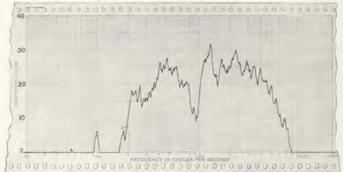
Plot of frequency response of a public-address system made on the graphic level recorder driving the frequency dial of the beat-frequency audio generator.
