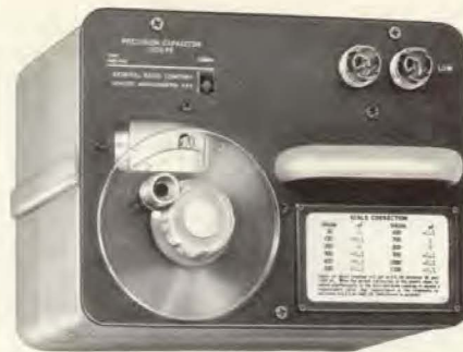
Two aluminum extrusions are strip-locked together to form the sides, heavy aluminum panel and bottom plate are added, and this precision capacitor is given the excellent shielding and trim appearance of the lab bench cabinet.
