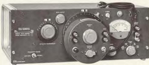
Type 1304-B Beat-Frequency Audio Generator driven by a Type 908-R96 Dial Drive, for use with an XY plotter.
