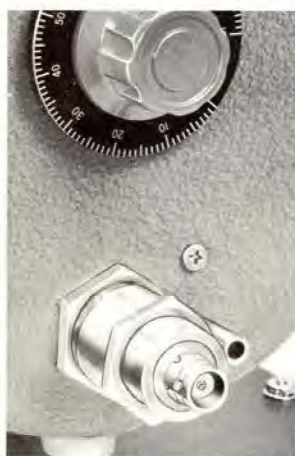
unit oscillator output connector adapted to type BNC with Type 874-QBJL
