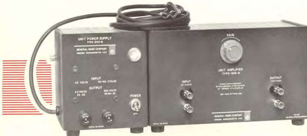
Type 1206-B Unit Amplifier with Type 1203-B Unit Power Supply.
