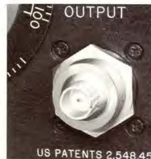
recessed Type 874 panel connector adapted to type TNC with Type 874-QTNJL
