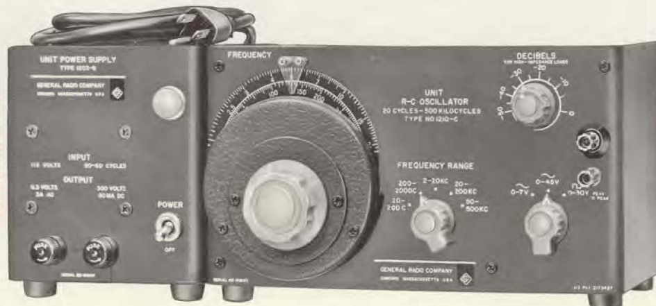
Type 1210-C Unit R-C Oscillator with Type 1203-B Unit Power Supply.
