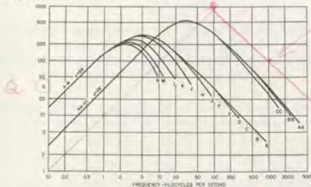
Figure 1. Q versus frequency for typical units.
