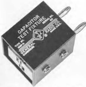
(Above) View of the Type 1691-A Capacitor Test Fixture. (Right) View showing disc-type ceramic capacitor inserted in fixture.
