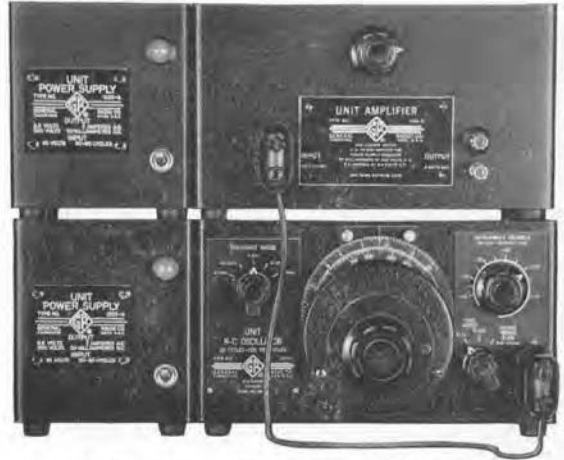
View of the TYPE 1206-A Unit Amplifier with the TYPE 1210-B Unit Oscillator. This combination delivers 3 watts over a range of 20 cycles to 50 kilocycles and 0.1 watt at 500 kilocycles.
