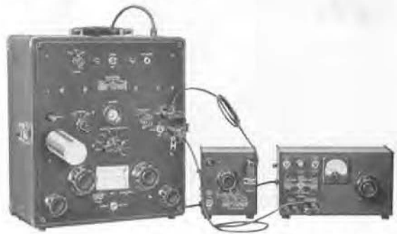
TYPE 1611-AS2 Capacitance Test Bridge used with the TYPE 1214-AS2 Oscillator to measure an electrolytic capacitor. The TYPE 1204-B Unit Variable Power Supply on the right supplies the d-c polarizing voltage.
