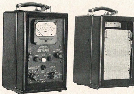
Type 1230-AE Electrometer and DC Amplifier with a recorder.
