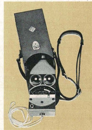
Sound-Level Meter in leather carrying case.
