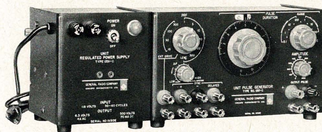
This Unit Instrument and power supply make a neat combination, with no wasted space. Chassis-mounted multipoint power connectors mate, and locking strips are supplied to make the union permanent, if desired.
