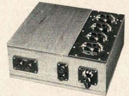
Type 216 Capacity Bridge 1920
