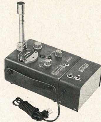
(Left) Microphone in the storage position (batteries automatically disconnected). (Center) The sound-level meter operated in its leather carrying case, microphone in the horizontal operating position. (Right) The sound-level meter ac-operated with the Type 1262-B Power Supply, which plugs directly into the base of the sound-level meter.
