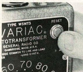
Overload protector, an important feature on portable models, is quickly reset from front panel.
