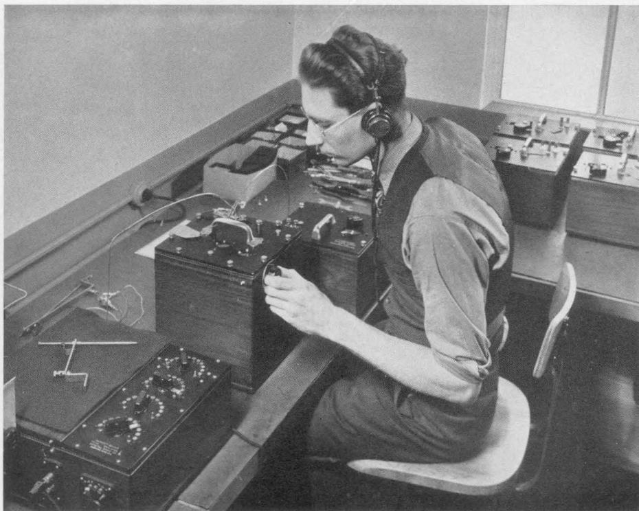
FIGURE 8. Calibrating a TYPE 722-F Precision Condenser
