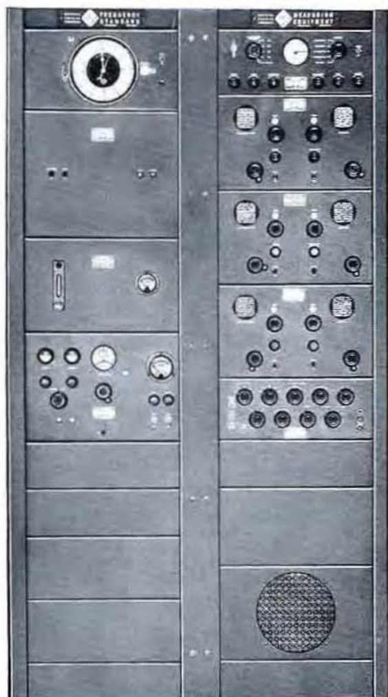
View of TYPE 1105-A Frequency Measuring Equipment with TYPE 1100-AP Primary Frequency Standard. The measuring equipment assembly is supplied with one floor-type relay rack, and the Type 1107-A Interpolation Oscillator mounts in the frequency standard rack, below the standard.
