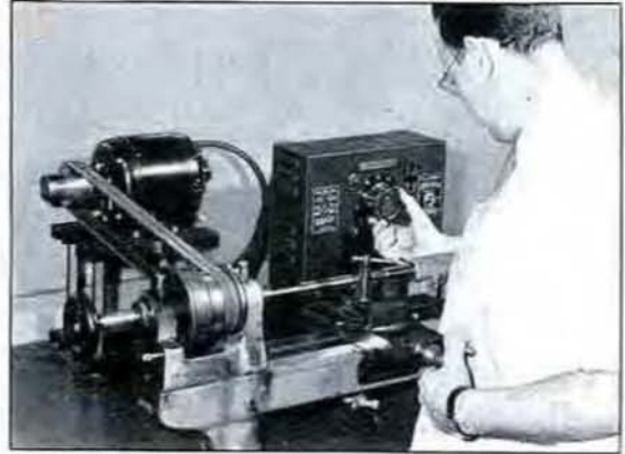
TYPE 1700-AI, Variac Speed Control in use on a bench lathe.
