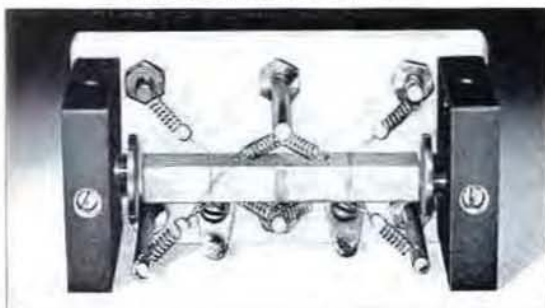
FIGURE 2. View of the Type 1100-A Quartz Bar used in Type 1100-A Frequency Standard, with cover removed, showing the spring suspension.
