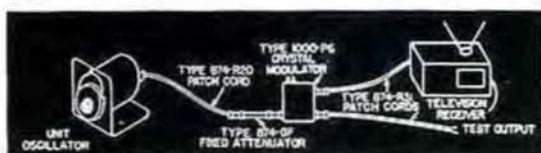
Functional diagram of the unit oscillator with video modulator to form a television signal generator.
