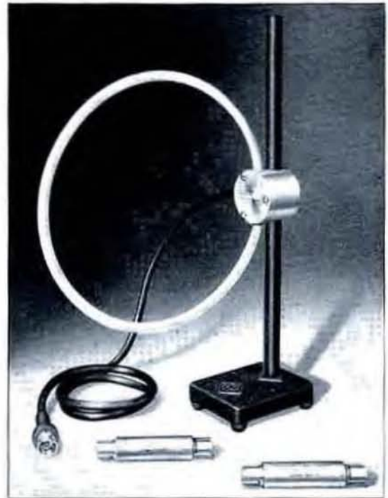
View of the Type 1000-P10 Test Loop, the Type 1000-P3 Voltage Divider, and the Type 1000-P4 Standard Dummy Antenna.
