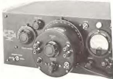
TYPE 1304-B Generator driven by a TYPE 908-R Dial Drive for use with an X-Y plotter.
