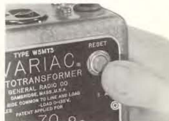
Overload protector, a new feature on portable models, is reset from front panel.
