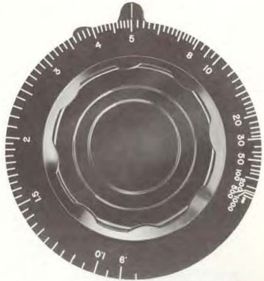
The Megohms dial of Type 544-B Megohm Bridge. The scale is approximately logarithmic over the main decade from 1 to 10.
