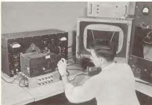
Production testing a crystal filter for i-f shaping. The filter operates at 13 Mc and has a 30-kc bandwidth. The sweep frequency is supplied by the TYPE 805-C Standard-Signal Generator, whose slow-motion dial is driven by the TYPE 1750-A Sweep Drive. Courtesy Hycon Eastern
