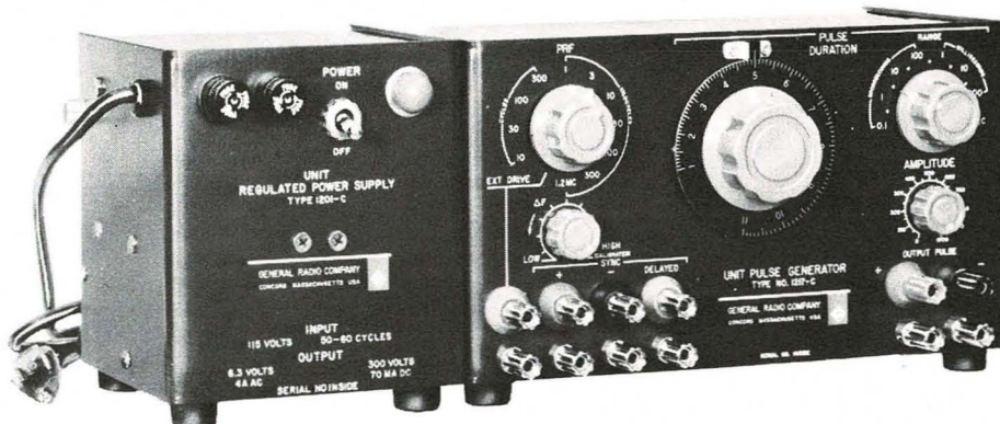
Unit pulse generator with power supply
