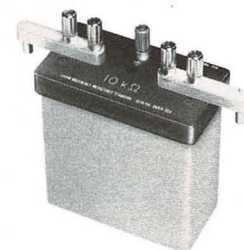
1444-B 10-k \Omega standard, for use with oil bath, shown removed from carrying case.
