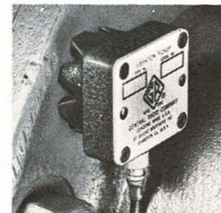
Vibration pickup with permanent-magnet clamp
