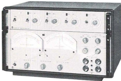
1654-Z1 Sorting System includes limit comparator for additional limits.
