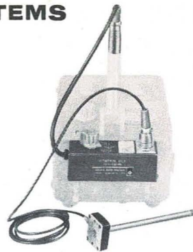
The 1560-P11B Vibration Pickup System with the 1551-C Sound-Level Meter.
