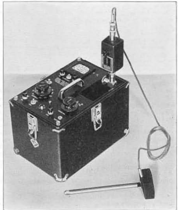
The vibration pickup and control box plug into the sound-level meter in place of the microphone, as shown here.
