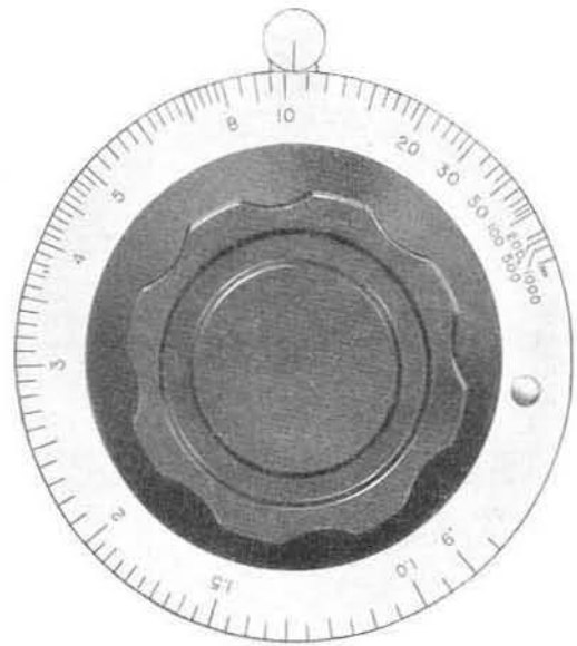
The MEGOHMS dial of TYPE 544-B Megohm Bridge. The scale is approximately logarithmic over the main decade from 1 to 10.
