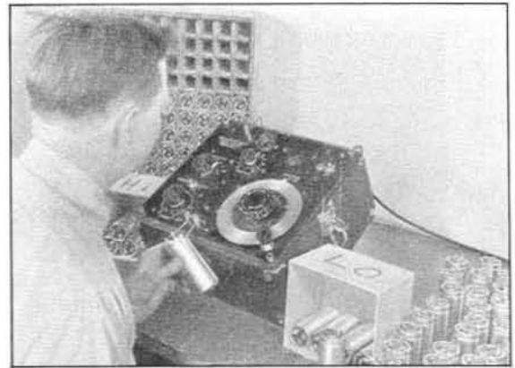
Production testing of electrolytic capacitors with the capacitance test bridge.
