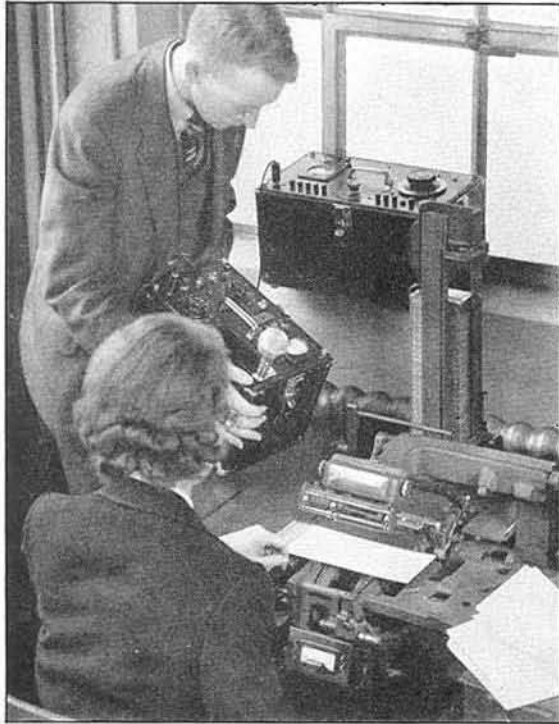
The TYPE 759-B Sound-Level Meter and the TYPE 760-A Sound Analyzer are useful for the study and analysis of office machinery noises (shown above is an automatic addressing machine) as well as for measurements on industrial machinery, operating household appliances, and other equipment.
