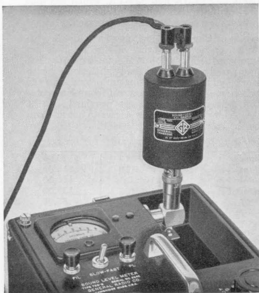
Figure 1. View of Type 1552-A Sound-Level Calibrator in operating position on microphone of Type 759-B Sound-Level Meter.
