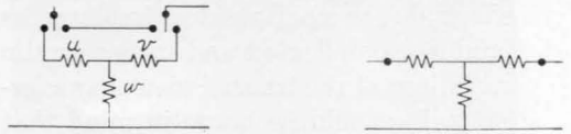
Figure 2. Elements of a T-pad, u and v series elements, w shunt element.
