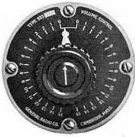
The TYPE 553 Volume Control is a fader. Left , the dial plate; right , the schematic diagram
