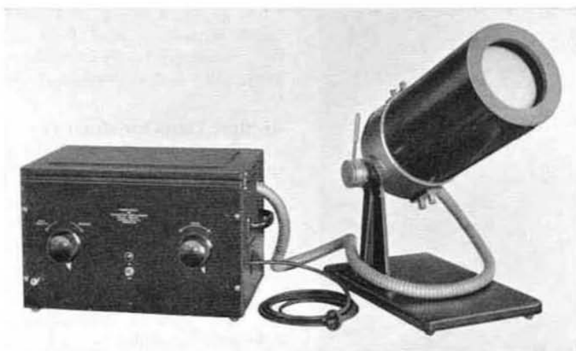
The General Radio Cathode-Ray Oscillograph for table mounting. At the left is the TYPE 496-BM Power-Supply Unit; at the right, the TYPE 497-A Tube Mounting containing the tube
