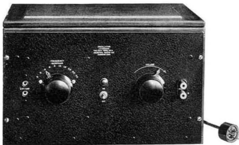
Operated entirely from the 110-volt alternating-current mains, the TYPE 508-A Oscillator delivers 10 frequencies between 200 cycles and 4000 cycles. This illustration shows TYPE 508-AM Oscillator
