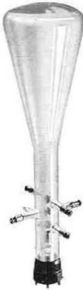
The tube used in the General Radio Cathode-Ray Oscilloscope
