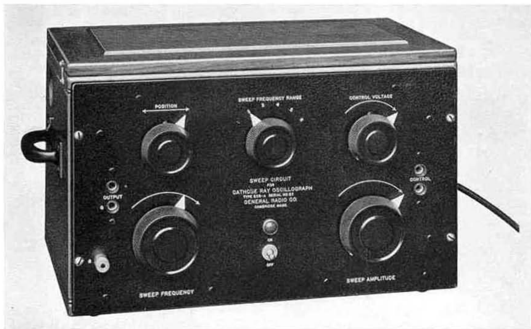
This sweep circuit supplies a linear time axis for the cathode-ray oscillograph. Linearity, wide frequency range, and a-c operation are its principal features
