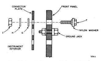
Figure 2-7. Removal of connector plate from front panel.
