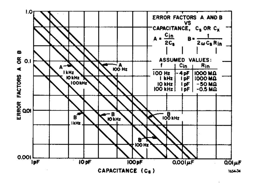
Figure 3-5. Factors A and B vs capacitance.
