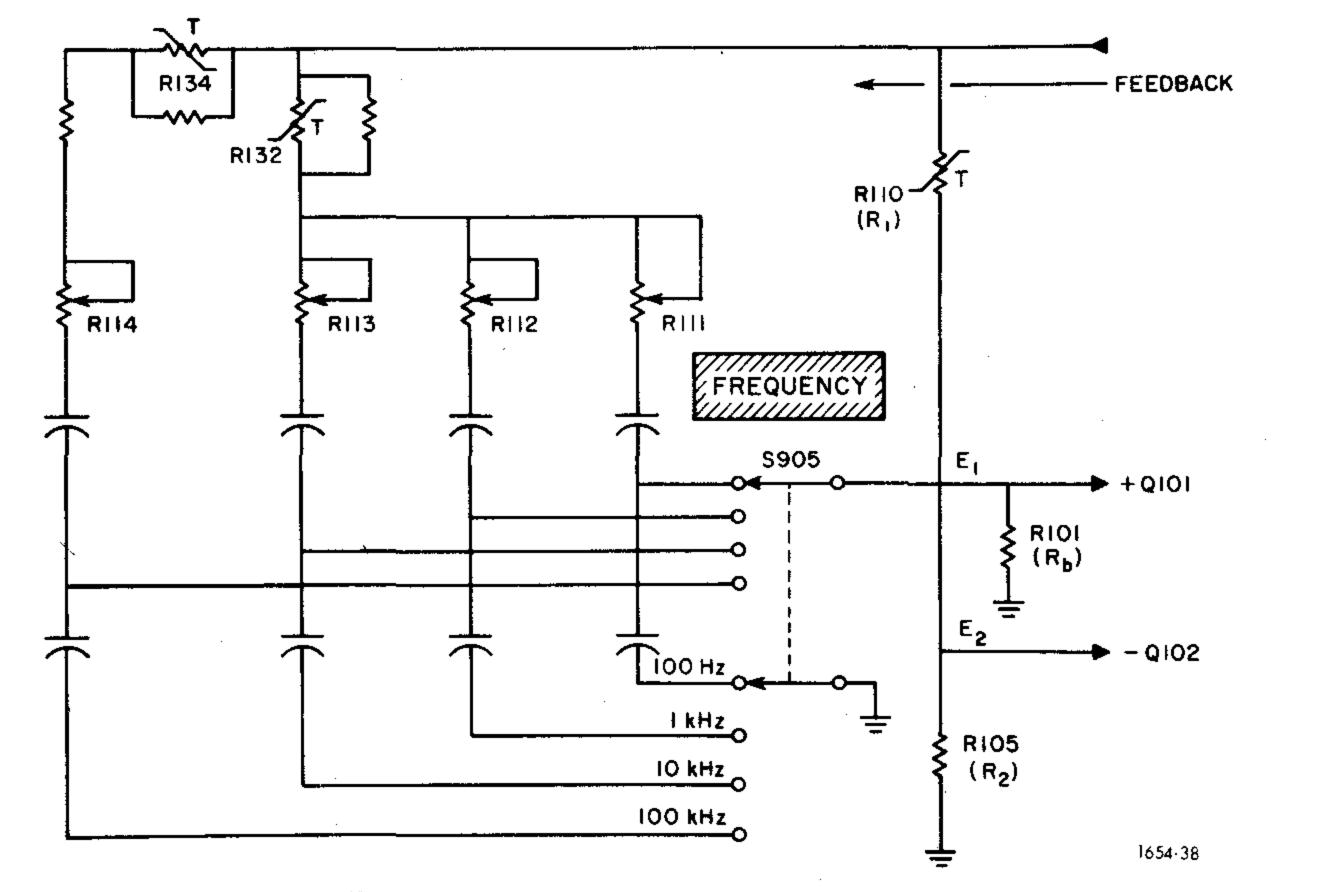
Figure 5-3. Bridge network schematic.
