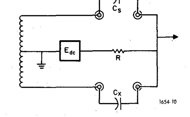
Figure 4-14. External bias (E<sub>dc</sub>) applied to standard and unknown capacitors.
