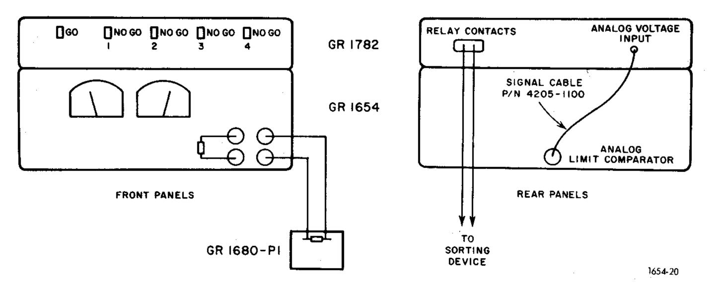
Figure 4-23. Typical test setup for high-speed selection and sorting of R, L, and C components.
