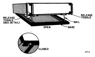
Figure 2-3. The 1654 tilted for better view of frontpanel controls and indicators.
