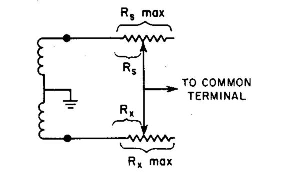
Figure 4-4. Setup for comparison of rheostats.
