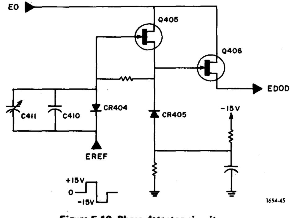
Figure 5-10. Phase-detector circuit.
