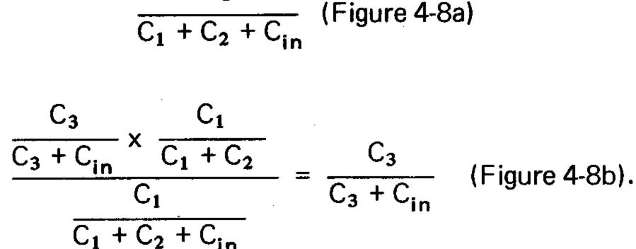
Another way of measuring input capacitance is to compare two known capacitors and calculate Cin:
