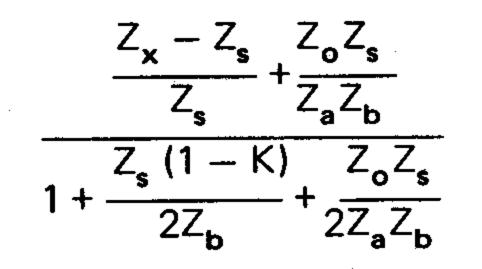
where:  $Z_o = output$  impedance of guard circuit  $\approx 1 \Omega$  in series with  $1 \mu$ F.
