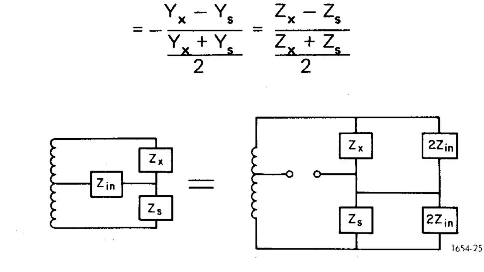
Figure 3-3. Alternate equivalent circuit of the loaded bridge circuit.
