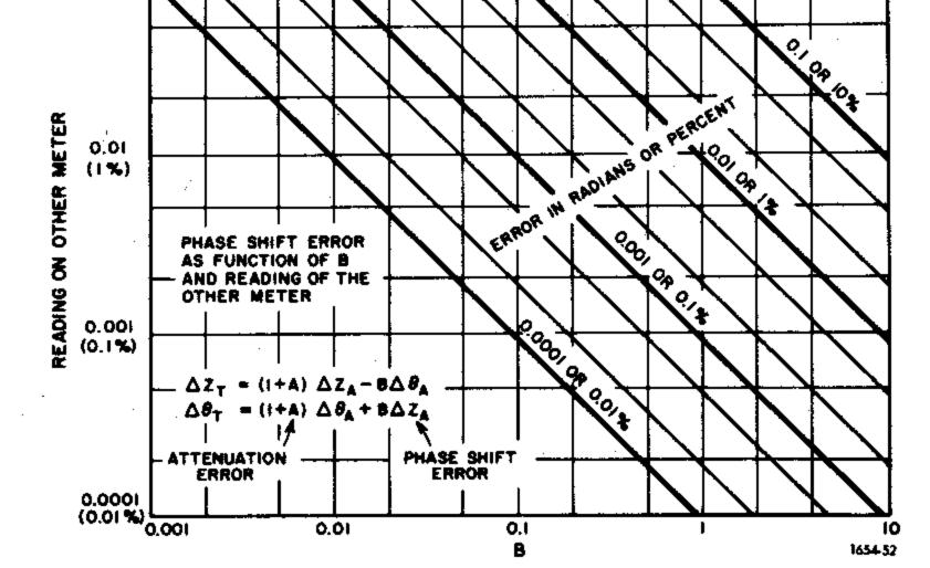
Figure 3-7. Phase-angle error as a function of B and  $\Delta Z$  range or magnitude error as a function of B and  $\Delta \theta$ .
