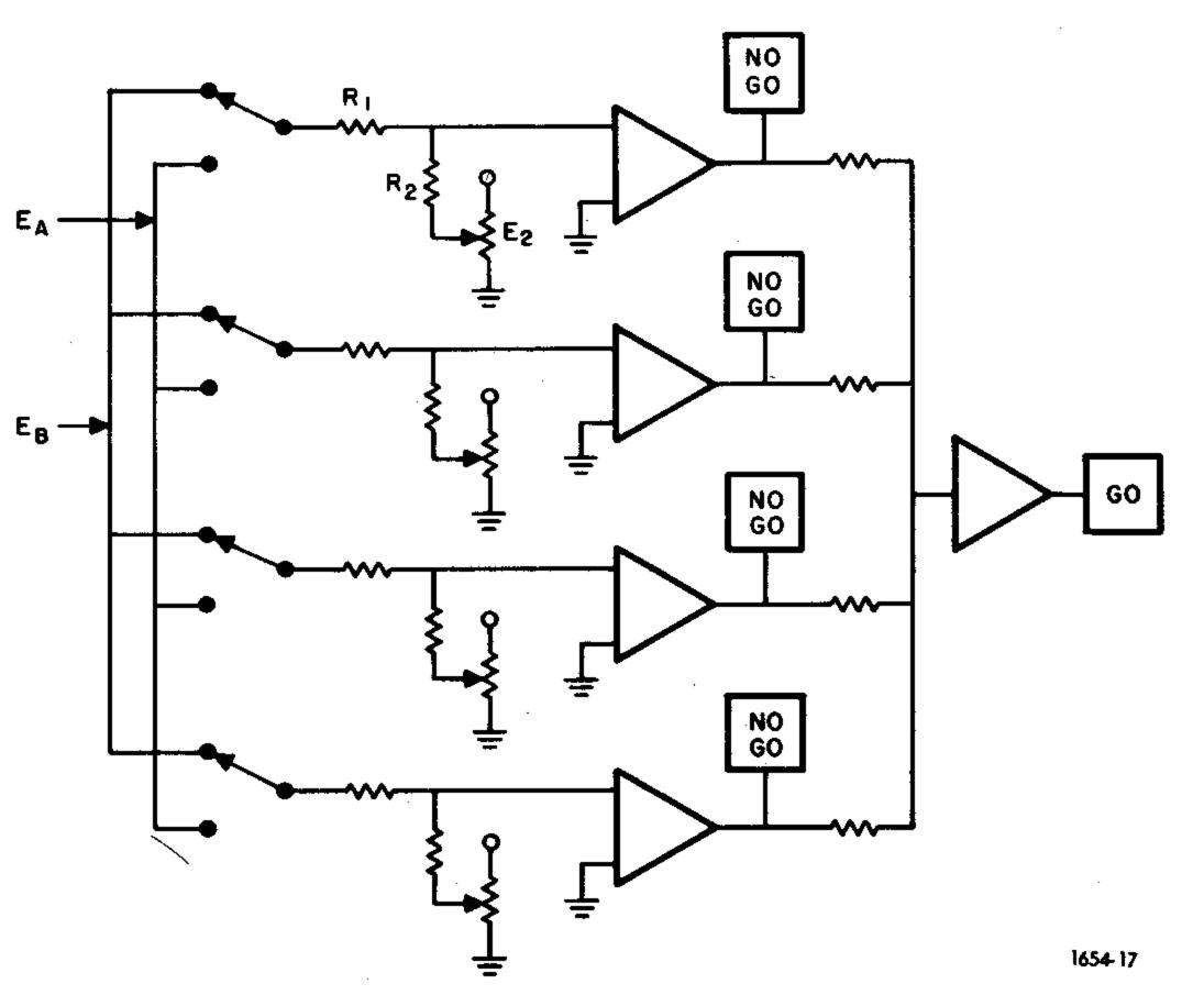
The 1782 can accept up to two inputs simultaneously in the form of analog voltages from 0 to ±10 V. For example, one input is the magnitude difference and the other the phase-angle difference. The source resistance of the input should be less than 100  $\Omega$ .
