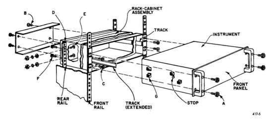
Figure 2-5. Relay-rack installation.
