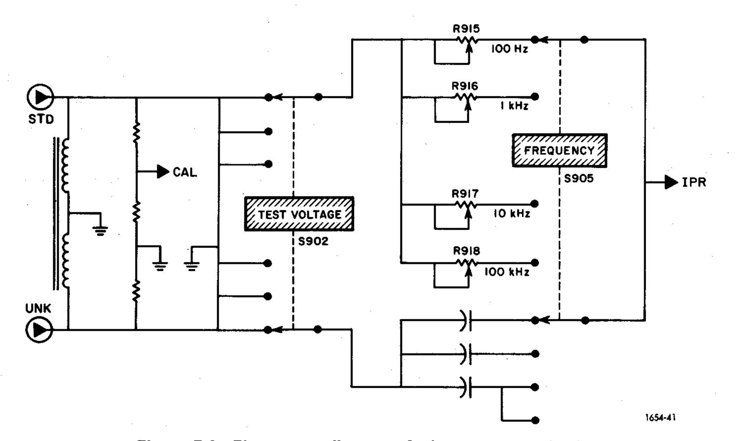
Figure 5-6. Elementary diagram of phase-converter circuit.
