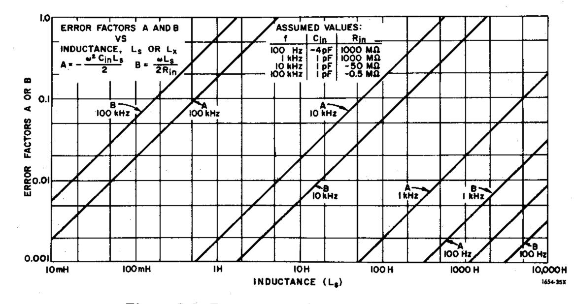
Figure 3-6. Factors A and B vs inductance.
