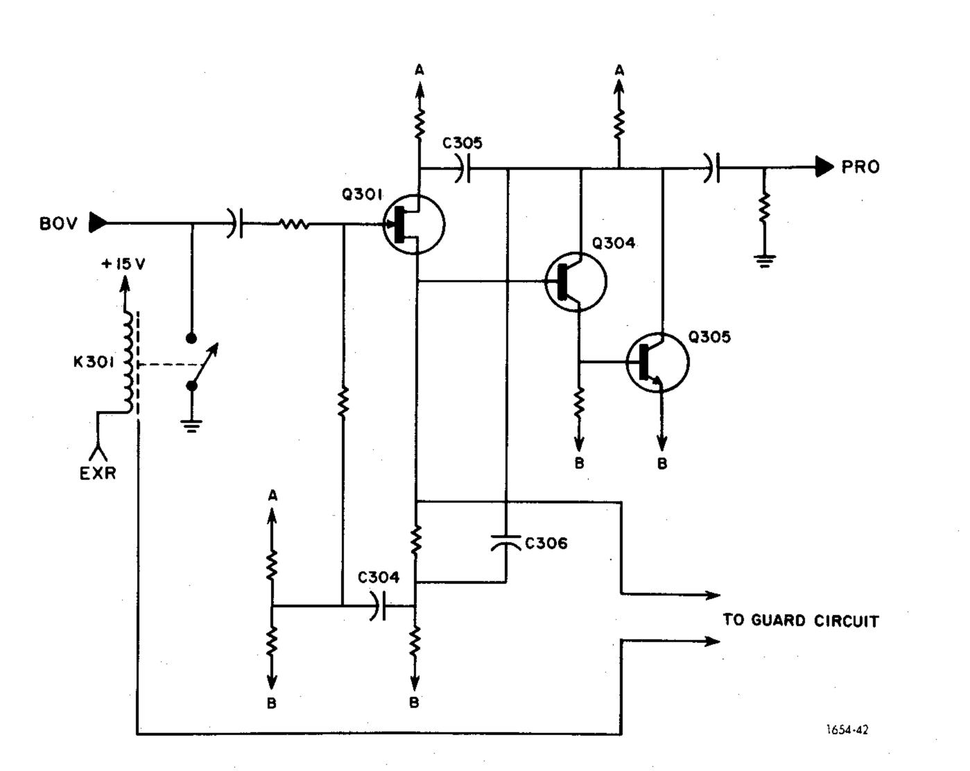
Figure 5-7. High-impedance amplifier used in the unbalance-amplifier circuit.
