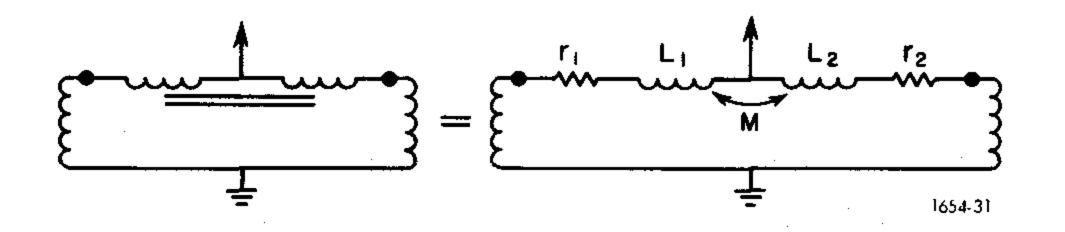
Figure 4-13. Measurements of balanced transformer windings.
