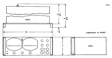
Figure 2-2. Dimensions of the relay-rack model 1654 Impedance Comparator.
