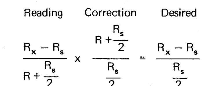
As an example, the correction for measuring resistance difference is given above. The resistors (R) need not be equal since it is possible to determine the difference and correct for it.
