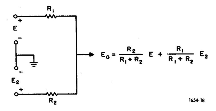
Figure 4-22. Comparison of input signal (E) with preset voltage  $(E_2)$  in 1782.
