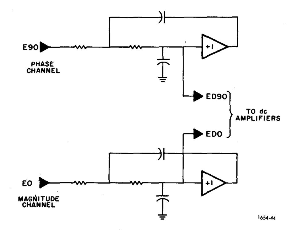
Figure 5-9. Block diagram of detector circuits.
