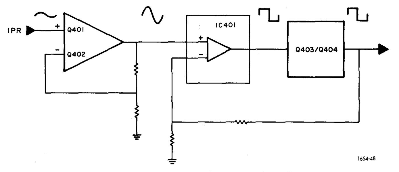
Figure 5-13. Square-wave, reference-signal circuit.
