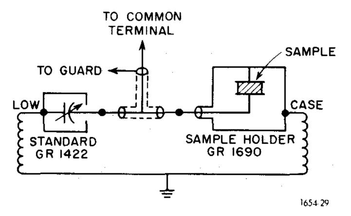
Figure 4-12. Measurement of dielectric samples using the 1690 Dielectric Sample Holder.
