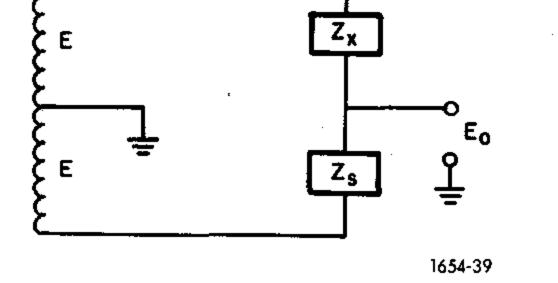
Figure 5-4. Basic bridge circuit.
