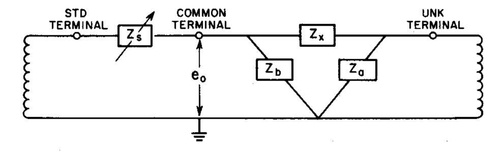
Figure 4-2. Direct impedance measurement using a variable standard.
