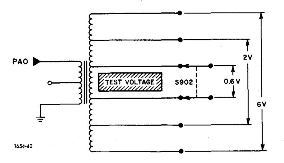
Figure 5-5. Bridge driver transformer.
