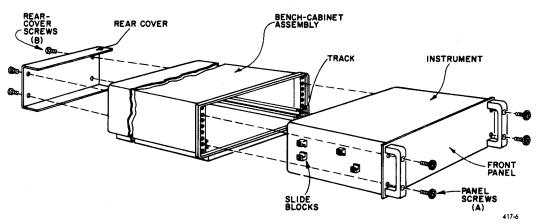
Figure 2-4. Cabinet removal and conversion for rack mounting.
