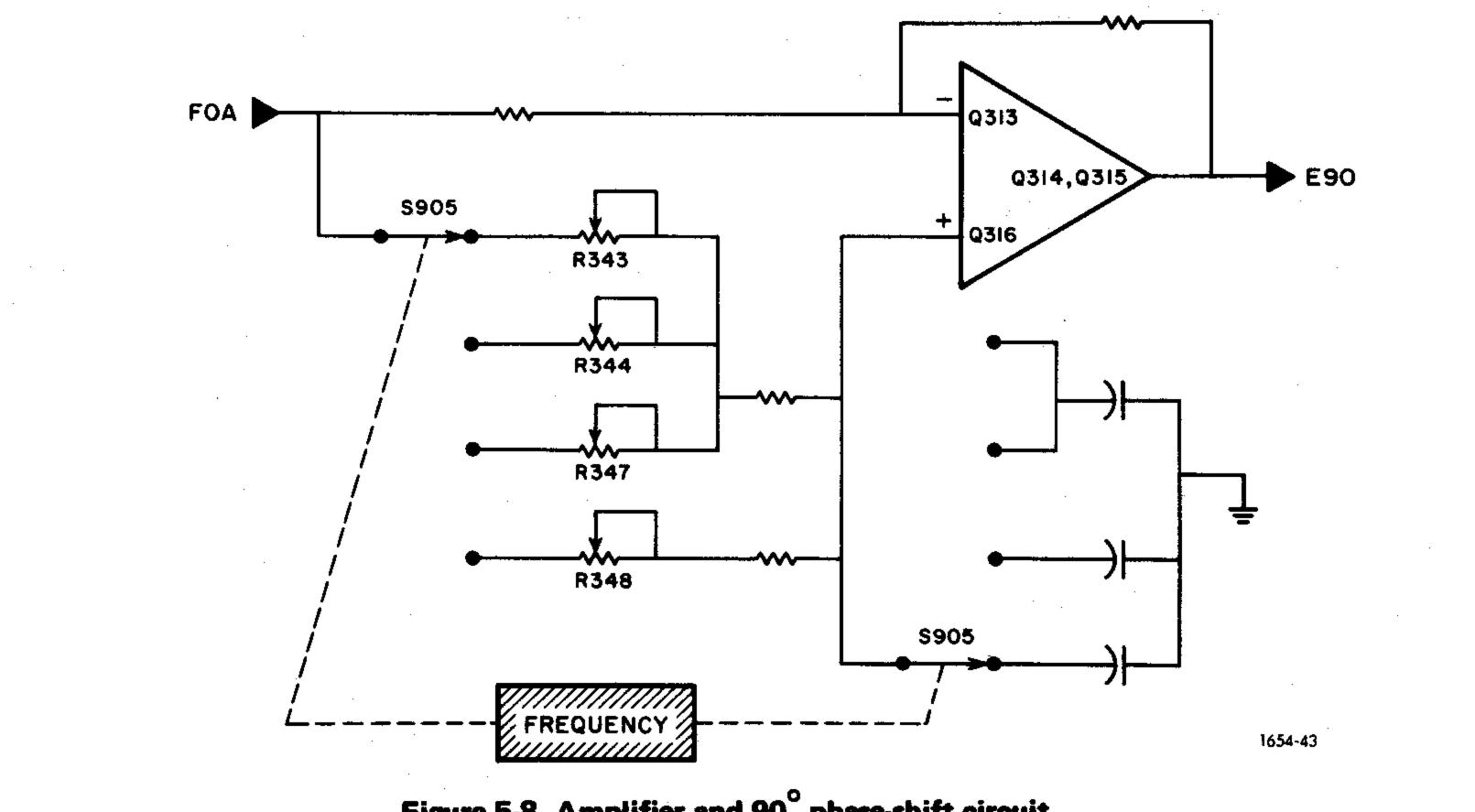
Figure 5-8. Amplifier and 90° phase-shift circuit.
