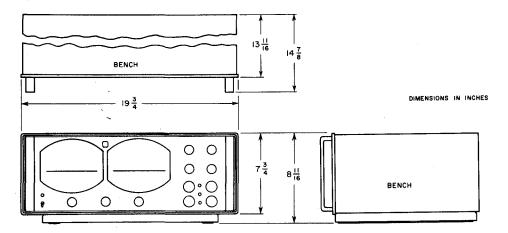
Figure 2-1. Dimensions of the bench model 1654 Impedance Comparator.
