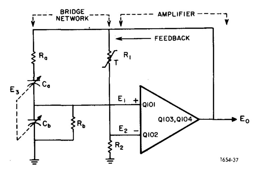
Figure 5-2. Diagram of RC Oscillator in the oscillator/ power amplifier circuit.
