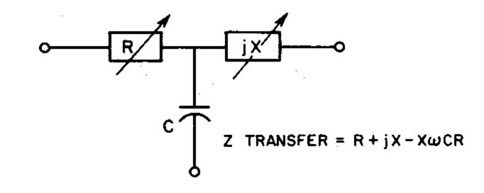
Figure 4-3. Possible error when series-connected variable standards are used.
