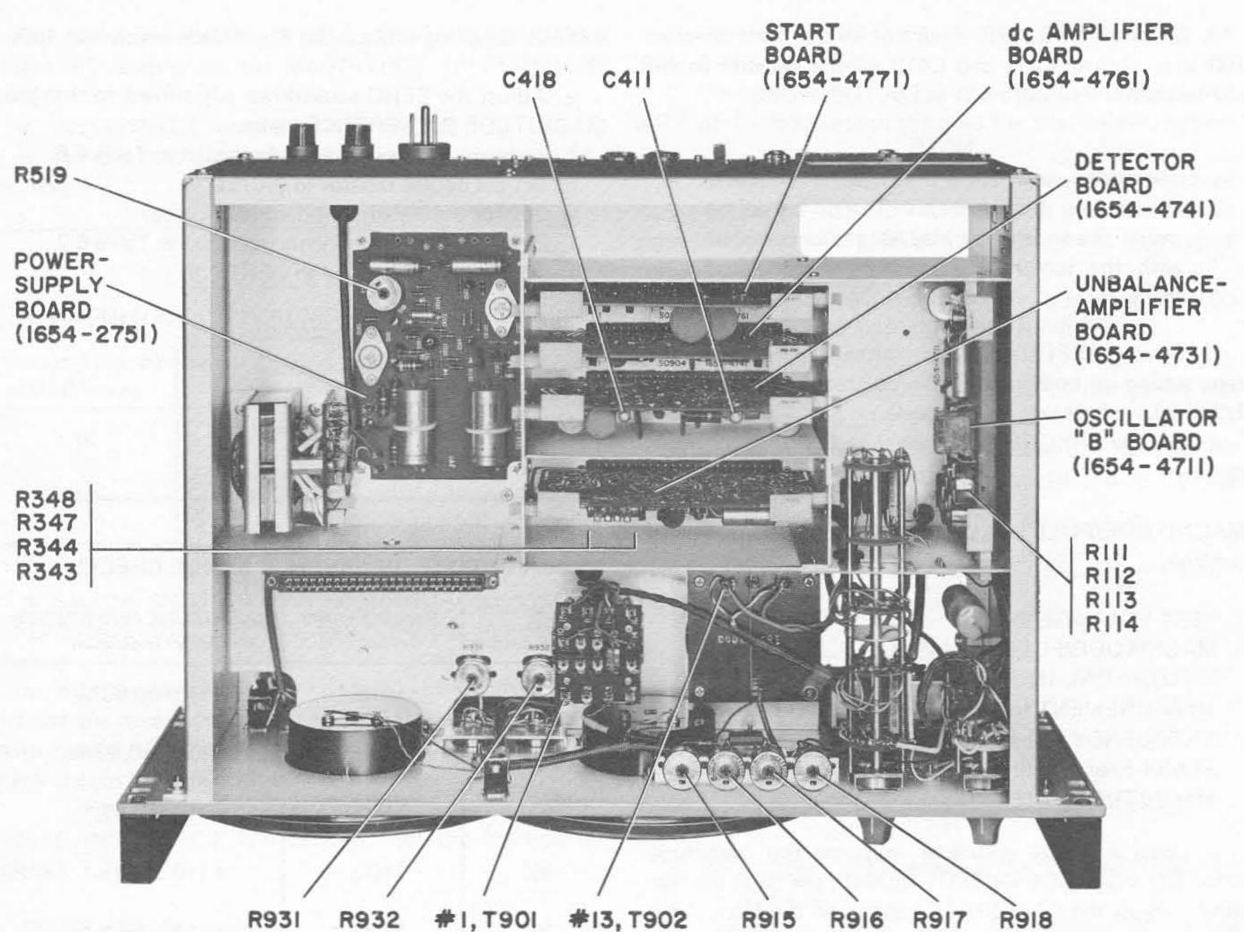
Figure 6-1. Top interior of 1654 Impedance Comparator.
