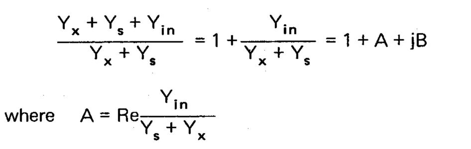
example, if the input resistance is 1000 M $\Omega$  (at such a frequency that the capacitance is negligible), there will be an error of approximately 1% when 20-M $\Omega$  resistors are measured.
