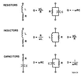
Figure 1-5. Definition of D and Q for series and parallel elements.
