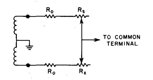
Figure 4-5. Preferred setup for comparison of rheostats.
