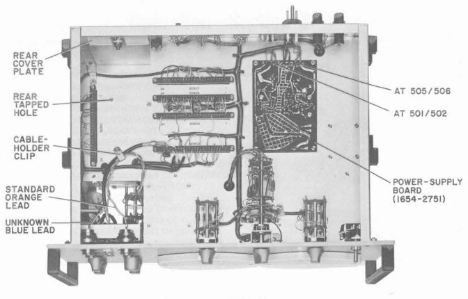
Figure 2-8. Bottom interior of 1654 with connectors installed in the front panel.
