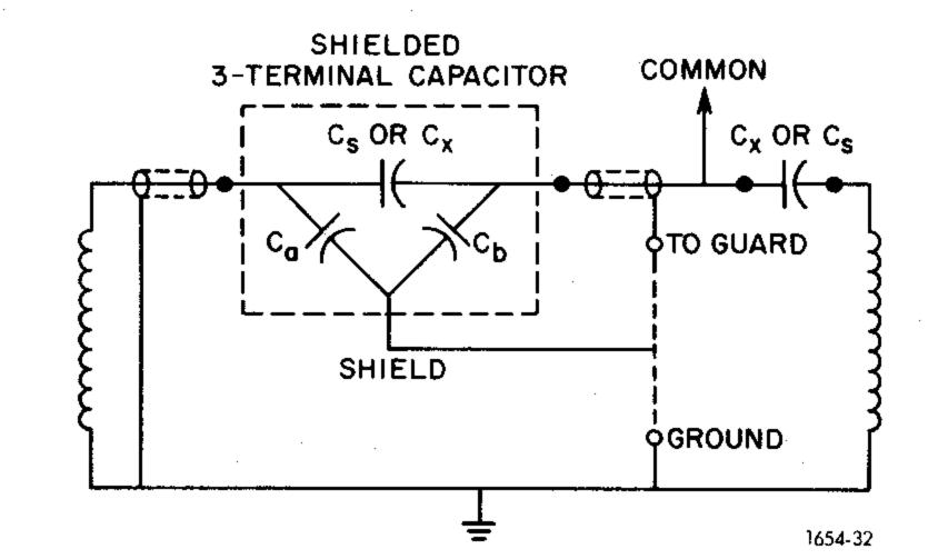
guard and the shield of the other lead (to the STANDARD or UNKNOWN terminal) should be grounded, if shielded wire is used. Note that these shields are not joined. Also, if the capacitor shield is guarded, it must be insulated from ground.
