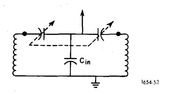
Figure 4-10. Comparison of ganged capacitors.
