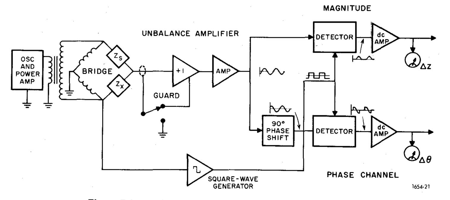
Figure 5-1. Block diagram of 1654 Impedance Comparator.
