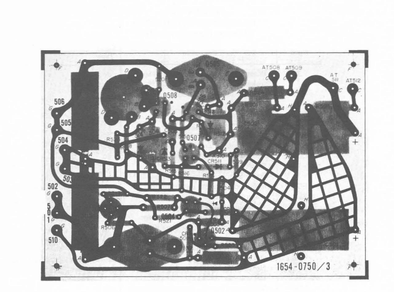
Figure 7-9. Power-supply etched-board assembly (P/N 1654-2751).
