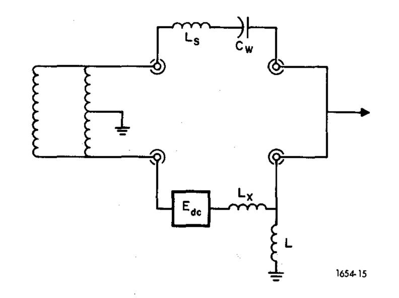
Figure 4-19. External bias (E<sub>dc</sub>) applied to unknown inductor only.
