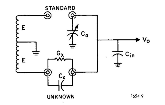
Figure 4-9. Measurement of small capacitance using an adjustable capacitor connected from the common (standard) terminal to ground.
