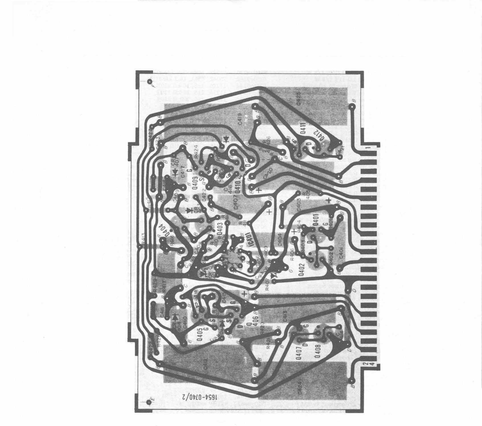
Figure 7-7. Detector-circuit etched-board assembly (P/N 1654-4741).
