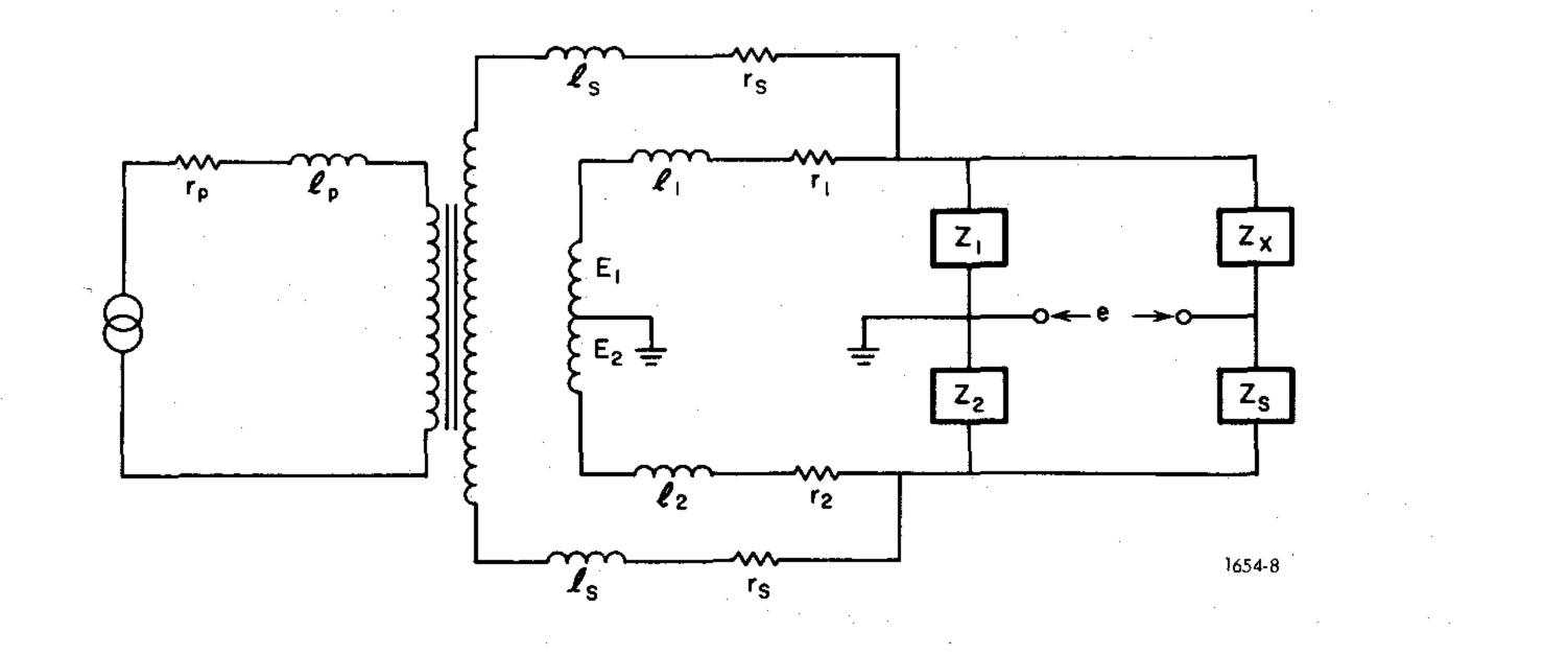
Figure 3-8. Equivalent circuit of a transformer.
