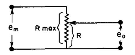
Figure 4-6. Potentiometer used as a divider.
