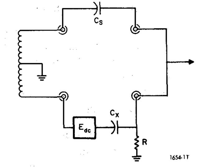
Figure 4-15. External bias (E<sub>dc</sub>) applied to unknown capacitor only.
