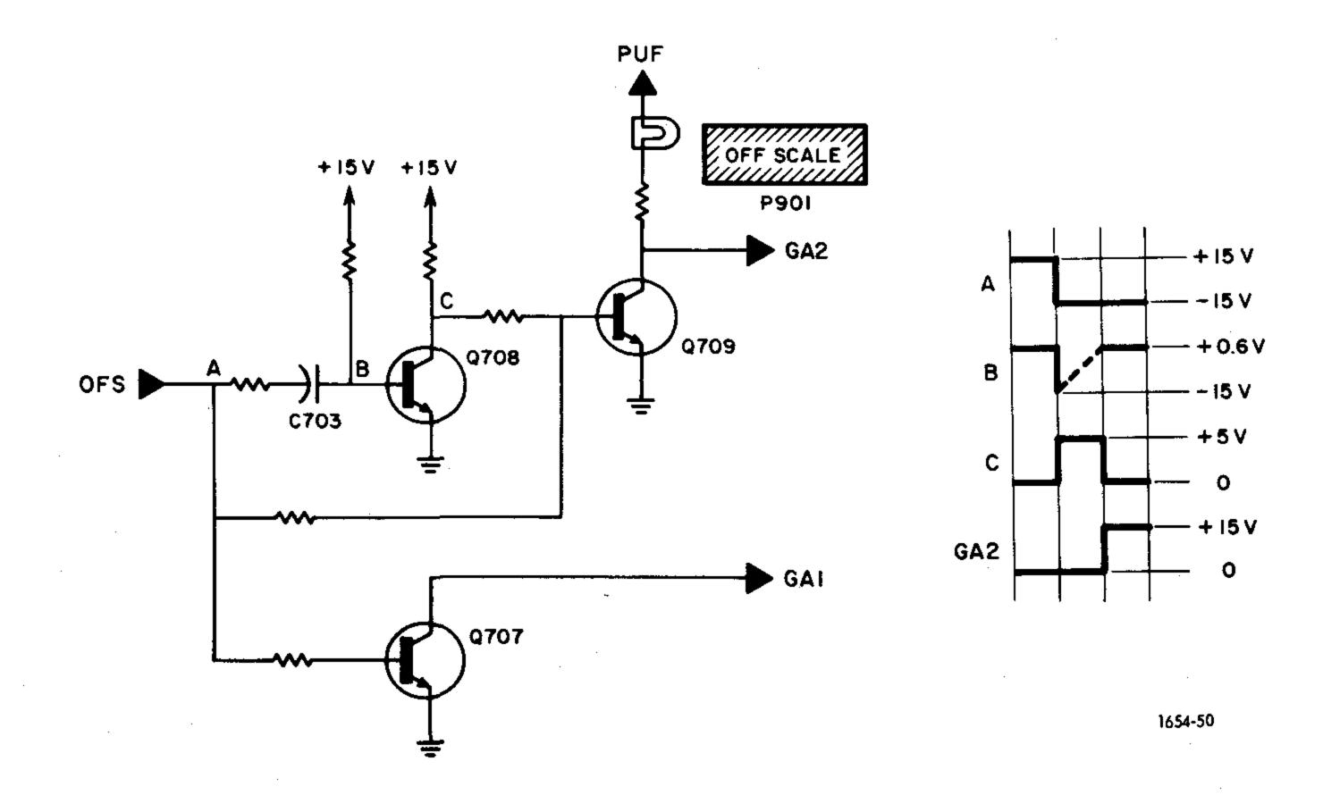
Figure 5-15. OFF SCALE and gate drivers.
