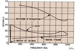
Typical noise figure, gain, and reverse attenuation characteristics of the VHF/UHF preamplifier.
