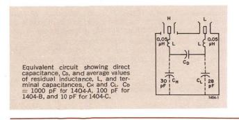
conveniently used to calibrate accurately a wide range of working standards in terms of a 1404 Reference Standard Capacitor. A single 1000- or 100-picofarad standard is also the only standard necessary to calibrate the bridge itself.
