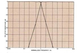
Low-pass and high-pass filter characteristics.
