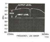
dBm and the subsequent change in gain observed. Since the measurement is automatic and the results are quickly obtained, displays of this type are very useful for tuning or otherwise adjusting wide-band circuits.
