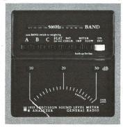
attenuator system is used (OPTI-RANGE). With this feature, you need only set a single range control for an on-scale indication. A second control is provided for situations where the automatic system may not be suitable, as with some measurements of transient signals.
