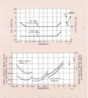
Performance. Upper: Specified sensitivity as input level for full scale indication, max gain, tuned. Lower: Typical noise level in terms of equivalent current and voltage sources.
