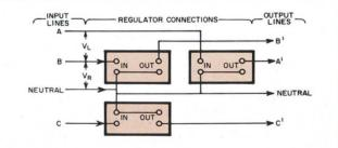
WYE The input voltage to each regulator ( $V_R$ , A, B, or C to neutral) is equal to the line-to-line voltage ( $V_L$ , A to B, B to C, or C to A) divided by 1.73. This reduces the input voltage requirements to about 58% of that normally required.
