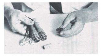
**5 Wires for a 2-Terminal Device?** Yes! The four-terminal (Kelvin) connections minimize lead-impedance effects and preserve the accuracy of the bridge *at the component* even with low-impedance unknown capacitors. And the fifth, or ground, terminal provides a similar safeguard with high impedances whose measurement might otherwise be affected by stray capacitance to ground. — See **GR Experimenter** for November-December 1969.
