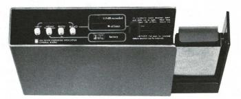
the accumulated percentage of noise exposure a worker has experienced . . . 100% being the maximum permissible in accordance with OSHA. A lamp on the Indicator lights in the event that 115 dBA has been exceeded at any time during the monitored period.
