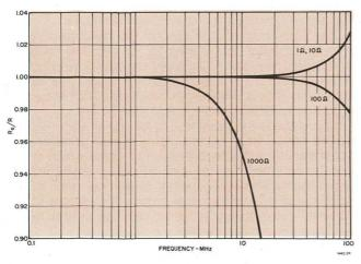
Typical ratios of effective ac series resistance to dc resistance, using a GR 900-WN connected to one end of the 1442 resistor.
