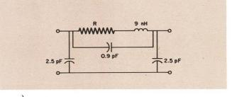
Equivalent circuit of a 1442 resistor shown with approximate values of capacitance and inductance.
