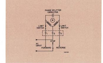
Schematic diagram of motor circuit
