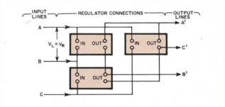
CLOSED DELTA The input voltage to each regulator (V<sub>R</sub>, A to B, B to C, or C to A) is equal to the line-to-line voltage (V<sub>L</sub>); i.e., V<sub>R</sub> = V<sub>L</sub>. The input range increases by slightly over 50%. Thus, the input range increases to  $\pm$ 7.5,  $\pm$ 15,  $\pm$ 31, and +37 -28% from the normal  $\pm$ 5,  $\pm$ 10,  $\pm$ 20, and +24 -18%, respectively.
