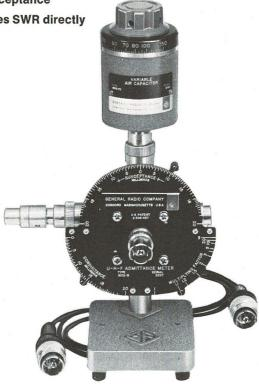
Versatile building block This null-type instrument measures complex impedance and admittance in coaxial systems and, as a reflectometer, will determine SWR, impedance magnitude, and reflection coefficient magnitude. It can be used to adjust a network to a predetermined admittance, to match one network to another, and to match antennas and other networks to 50-ohm circuits.
