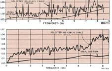
Typical SWR performance of a single Type 900-C9 Connector on an "infinite" length of RG-214/U cable and on an "ideal" section with the same diameters.
