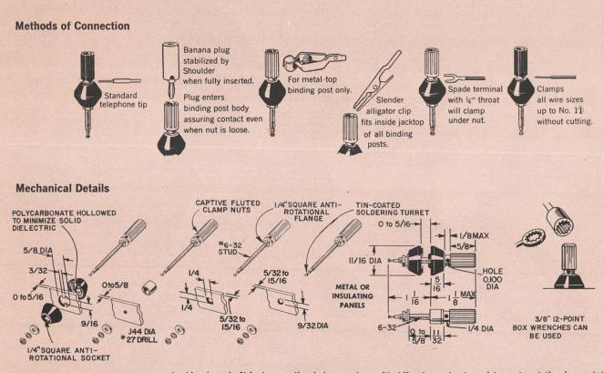
Locking keys in 5%-inch mounting holes can be omitted if only moderate resistance to rotation is needed.
