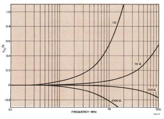
Typical ratios of effective ac series reactance to dc resistance, using a GR 900-WN connected to one end of the 1442 resistor.
