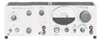
The 1232-A Tuned Amplifier and Null Detector and the 1311-A Audio Oscillator have been combined for use with audio-frequency bridges and other null-balance devices. This assembly occupies a minimum of bench space and is supplied with removable panel extensions, which adapt it for rack mounting.
