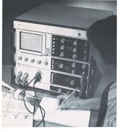
**Tailored capability** The 1710 is a sophisticated, yet simply operated system for accurate measurements of magnitude, phase, and group delay of either of two signals relative to a third reference signal; impedance and immittance measurements are equally simple. The analyzer operates over a broad swept-frequency range of 400 kHz to 500 MHz and a wide dynamic range of 115 dB in either 50- or 75- $\Omega$  systems.
