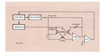
to be trimmed in closed-delta configurations and thus eliminates the need to break a resistor chain or to bond resistors together after trimming. Unguarded 4-terminal Kelvin connections and simple 2-terminal measurements are also possible.
