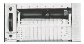
**Conveniences standard** All plug-ins feature remote programmability, a variety of inputs and outputs to synchronize recorder operation with that of other instruments, and a choice of several potentiometers with dynamic ranges from 10 dB to 100 dB to tailor the instrument to your specific requirement.
