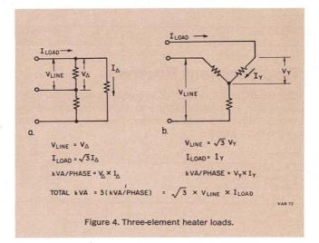
configuration in which the maximum voltage allowed, 140 V, will be applied to each unit in the assembly, thus preventing added voltage from being developed for the load. To get overvoltage capability, find, in the table, the next model that is wired in an open delta and has adequate "maximum current" rating: The W30HG2. A quick look at larger open-delta assemblies confirms that this is the least expensive choice.
