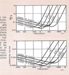
**Dissipation Factor:** Not greater than 0.001, 0.0005, and 0.0003 for capacitances of 100 to 1000 pF, 1100 to 2000 pF, and 2100 pF to 1.1110  $\mu$ F, respectively.
