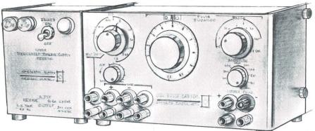
Unit pulse generator with power supply
