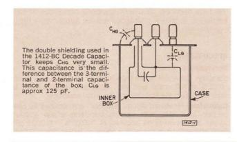
styrene dielectric used in the decade steps is necessary for applications requiring low dielectric absorption and constancy of both capacitance and dissipation factor with frequency.
