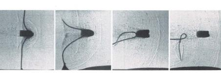
Strobe shadowgraph shows a .22 caliber bullet striking and being cut in two by a steel wire — the supersonic whip of the wire end is clearly visible. Separation of the four images is achieved by flashing the strobes at intervals of 40 microseconds.
