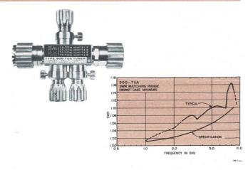
**Electrical:** IMPEDANCE: 50.0  $\Omega$ . INPUT POWER: <1 W continuous, or <500 W peak with <1 W average. DC RESIST-ANCE: 50.0  $\Omega$ <sup>±</sup>0.3% when terminated in 50.0  $\Omega$ . Mechanical: DIMENSIONS: 3.75 in. (95 mm) long. WEIGHT: 0.7 lb (0.4 kg) net.
