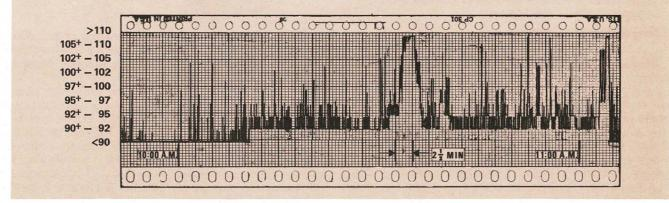
An actual strip-chart record made using the MFE accessory recorder with the Noise-Exposure Monitor in the course of an hour at a noisy work station. The cumulative noise exposure at this station was 110% for the 8-hour day. From the plot it can be readily determined that 13% of the permitted daily exposure occurred between 10:33 and
