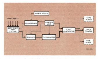
Simplified block diagram of automatic leakage-current measurement system.
