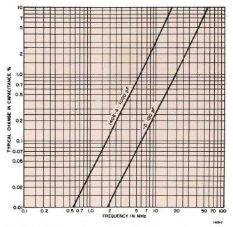
Typical percent increase in capacitance with frequency of 1406 Coaxial Capacitance Standards.
