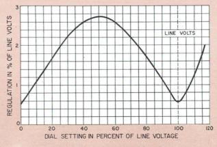
Typical regulation curve with normal rated current.
