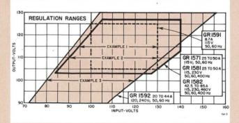
Information is shown for 115- and 120-V, 60-Hz models. For 230-V models, multiply voltages and divide current ratings by 2 (for 460-V models, by 4). The regulation range is slightly less for 400-Hz models but is significantly greater in some three-phase applications. (See Three-Phase Selection, three-wire inputs.) More detailed information, particularly current ratings, is given with the descriptions of the individual regulators.
