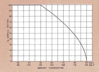
Figure 2. Variac autotransformer derating versus ambient temperature.
