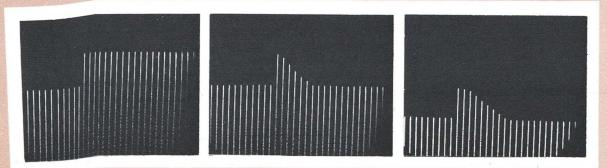
Oscillograms of line-voltage peaks show response speed of Variac® automatic voltage regulators: left, 2% step change in line voltage; center and right, resulting output transients for 1581 and 1582 Regulators, respectively.
