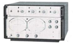
1654-Z1 Sorting System includes limit comparator for additional limits.
