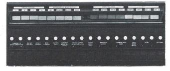
126 COMPONENT AND NETWORK TEST SYSTEMS File Courtesy of GRWiki.org allows any one of four optional pushbutton-selected tests to be performed, including the ripple rejection of voltage regulators, 10-k $\Omega$ -loaded gain of operational amplifiers, and any two other custom tests you may need for your particular circuit. A burn-in period can also be introduced after the initial current tests, which provides a one-second interval under power to allow the device junctions to stabilize.
