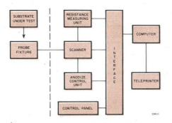
Basic elements of GR "RATS" Computer-Controlled System.
