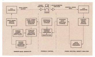
Functional block diagram of vibration control system.
