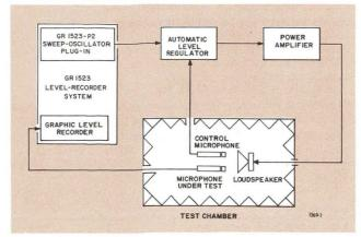
Typical measurement system using 1569.
