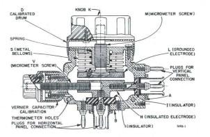
A precision micrometer screw, M, with large instrument knob, K, drives the movable grounded electrode, L, with respect to a fixed, insulated electrode, H. An accurately divided drum, D, indicates the electrode spacing. The micrometer screw is electrically shunted by a metal bellows, S, to assure a positive, low-resistance connec-
