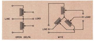
Consider the simplest cases where a single Variac unit is used in each arm. In the **wye** configuration, the full line-to-line voltage is not imposed on each unit, rather it is  $1/\sqrt{3}$  or about 58% of the voltage. Thus a 240-volt line will impose about 138 volts on each unit. However, each unit supplies the full line current to the load through its brush. In the **open delta**, the input to each unit is the full voltage from the line and each unit must supply the full line current.
