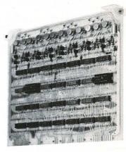
**32 inputs, 63 outputs** This assembly contains 7 BCD-to-decimal display tubes, 6 ten-position switches, an eight-
