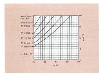
Power derating vs impedance setting and frequency. All 48 impedance settings are represented, as n = 0, 1, 2  $\ldots$  7.
