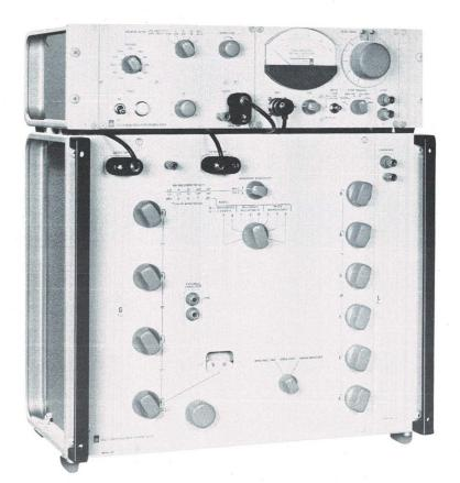
1660-A Precision Inductance-Measuring Assembly includes 1632-A Inductance Bridge, 1311-A Oscillator, 1232-A Tuned Amplifier and Null Detector.
