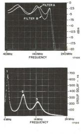
**High-attenuation filter response** This double exposure demonstrates the ease with which wide-dynamic-range measurements can be made. With normal gain, the entire response characteristics of the notch are not visible. But, by the simple flick of a switch, an additional 20-dB
