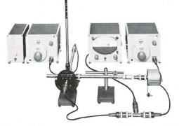
The Admittance Meter assembled for component measurements, with unit oscillator and 1241 Detector. A line stretcher (Type 874-LKL) connects the component mount to the unknown terminal of the Ad-mittance Meter.
