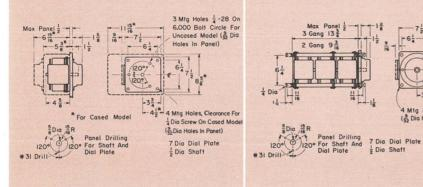
**Dimensions Ganged Uncased** Types W20G2, W20G3, W20HG2 and W20HG3
