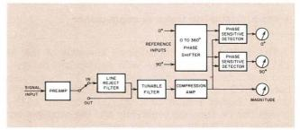
${<}30~\text{nV}\times\sqrt{\text{bandwidt}_{Hz}}$  at 1 kHz with input impedance of 70  $M\Omega\#500~\text{pF}.$  MONITORED by magnitude, in-phase, and quadrature meters; phase-sensitive detectors contain time-constant variable from 0.1 to 10 s in 5 steps.
