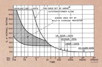
Figure 1. Short-time overload characteristic of Variac autotransformers with line-voltage connection.
