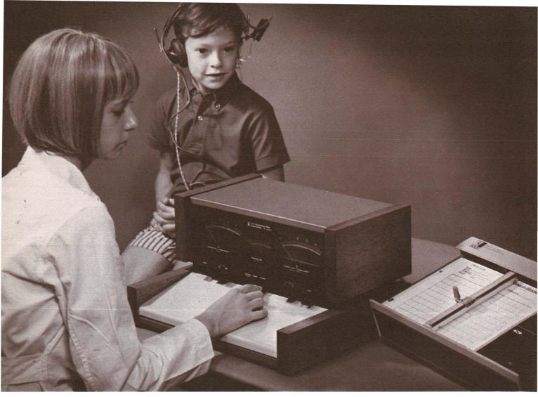
1720 Otoadmittance Meter as used in measurement of middle-ear function.
