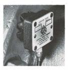
Vibration pickup with permanent-magnet clamp
