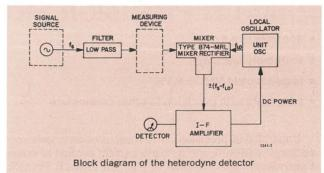
The system Each 1241 consists of an 874-MRAL Mixer, 1236 I-F Amplifier, 874-G10L 10-dB Pad, and 874-EL-L 90° EII , plus an oscillator and filter. For maximum shielding, components are equipped with locking GR874® connectors (which can be used interchangeably with the nonlocking type).
