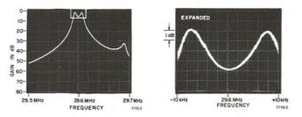
In this example, the characteristics of a crystal filter with a nominal center frequency of 30 MHz are first checked with a frequency resolution of 20 kHz per division and a magnitude resolution of 10 dB per division. A more detailed analysis is then made at 2 kHz per division to provide greater resolution around the center frequency. The measurements were made with a 50- $\Omega$  Transmission Tee.
