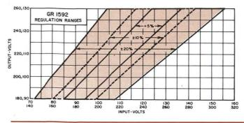
OUTPUT LEVELS V<sub>o</sub>, for specified regulation: See curves. Examples: ±20% model, 90 <V<sub>o</sub> < 130 V for input variation of 104 to 108 V; 100 <V<sub>o</sub> <120 V for 96 to 120 V; ±5% model, 113 <V. <117 V for 112-to-118 V input variation.
