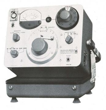
30-dB attenuation at one-half and twice the selected frequency. One-tenth-octave characteristic has at least 40-dB attenuation at one-half and twice the selected frequency. Ultimate attenuation is 70 dB or greater for both characteristics. For both bandwidths, peak response is uniform  $\pm 1$  dB from 5 Hz to 10 kHz and  $\pm 1.5$  dB from 2.5 Hz to 25 kHz. An *all*-pass, or flat, characteristic is also included.
