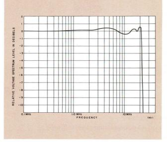
Typical spectrum of 1383 Random-Noise Generator output; energy-per-Hz bandwidth vs frequency.
