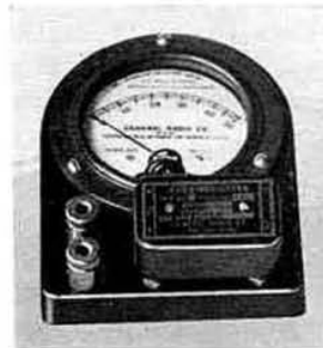
A TYPE 588-AM Direct-Current Meter showing how a TYPE 493 Thermocouple or a TYPE 492-A Oxide Rectifier can be plugged in
